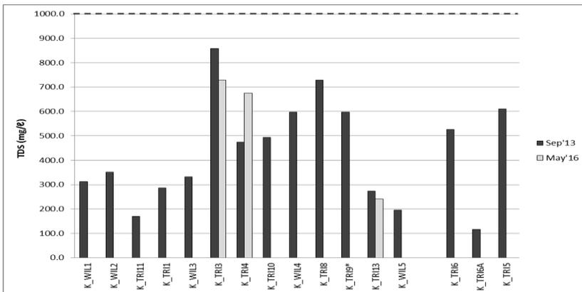
Figure 5: Total Dissolved Salts concentrations measured in August/September 2013 and selected points in May 2016 (dashed lines indicate guideline values, \* dry during the May 2016 survey)
