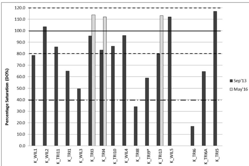
Figure 9: Percentage saturation (DO%) recorded during the August/September 2013 survey and selected points in May 2016 (dashed lines indicates target values, solid line indicates saturation and dot-dash line indicates lethal limit, \*site dry during the May 2016 survey)
