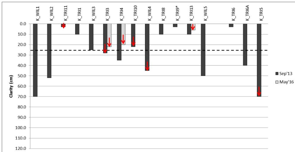
Figure 12: Secchi Disk depths recorded during the August/September 2013 survey and selected points in May 2016 as an indication of clarity (dashed line indicates low turbidity, arrows indicate 'more than' values, \*site dry during the May 2016 survey)
